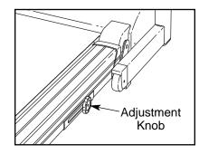
knob counterclockwise. To decrease the firmness, turn the knob clockwise. Note: The faster you run on the treadmill, or the more you weigh, the firmer the walking platform should be.
